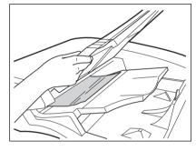
6 Open the original exit tray and remove any misfed originals.
